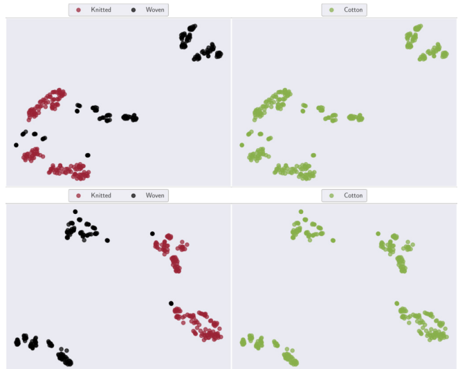
Fig. 6: Effect of splitting construction method on Cotton samples. t-SNE plot of measurements obtained from the active (top row) and passive (bottom row) arms during pulling Cotton samples.
